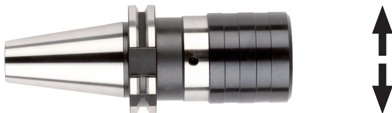
**Radial float** – allows for slight misalignment of the machine spindle axis and hole axis prior to tapping. This is not recommended manufacturing practice and should be avoided.
